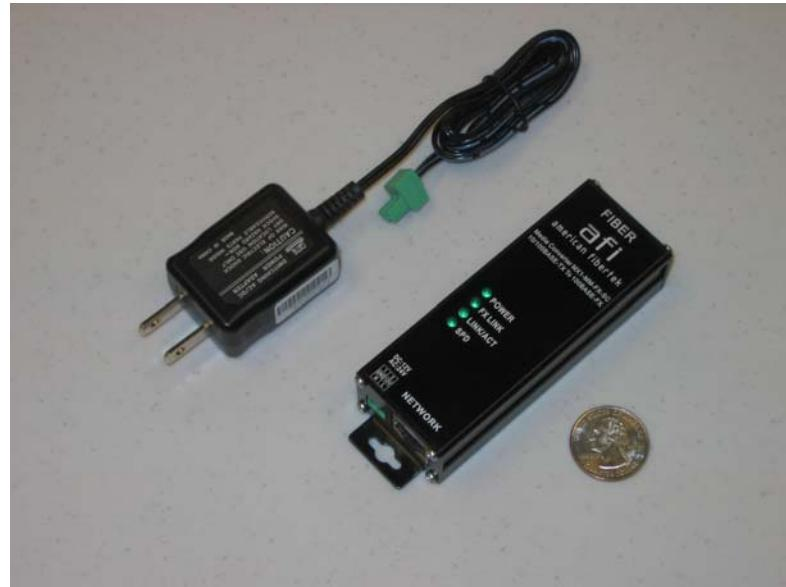
The American Fibertek MX1 Series transmits and receives 10/100 BaseT Ethernet signals at the RJ45 port and optical 100 Base-FX over 2 multimode fibers. The system is comprised of two units forming a point-to-point communications link.
